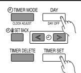
Press the DAY (DAY OFF) button and SET button simultaneously for 2 seconds or more to activate the child lock function and lock all buttons on the remote controller. Press the buttons again for 2 seconds or more to deactivate the child lock function.
