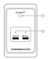
① **ON/OFF lamp** (lit when unit is operating; unlit when unit is not operating)
