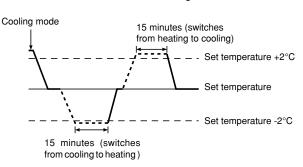
Because the room temperature is automatically adjusted in order to maintain a fixed effective temperature, cooling operation is performed a few degrees warmer and heating operation is performed a few degrees cooler than the set room temperature once the temperature is reached (automatic energy-saving operation).
