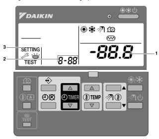
1 Press the <sup>™</sup> button for a minimum of 5 seconds to enter FIELD SET MODE.
